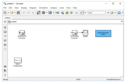
The new untitled model, with the default solver set to VariableStepAuto, contains a Solver Configuration block, a Simulink-PS Converter block, and a PS-Simulink Converter block connected to a Scope block.
