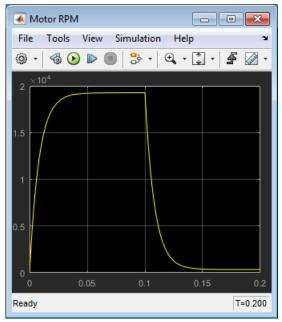
For the first 0.1 seconds, the motor has no external load, and the speed builds up to the no-load value. Then at 0.1 seconds, the stall torque is applied as a load to the motor shaft. Zooming in on the Motor RPM scope shows that the model matches the manufacturer parameters for no-load speed and stall torque.
