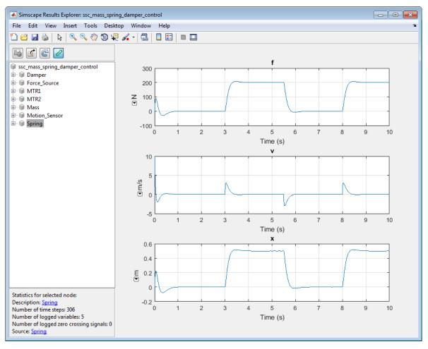
**3** Expand the Spring node and select node x. The right pane displays the spring deformation data plotted over time.
