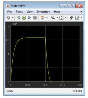
3 Try varying the load torque to find the maximum torque at this reduced voltage. Open the Step Input subsystem and double-click the Step source block. Enter different final values for the input signal and rerun the simulation.
