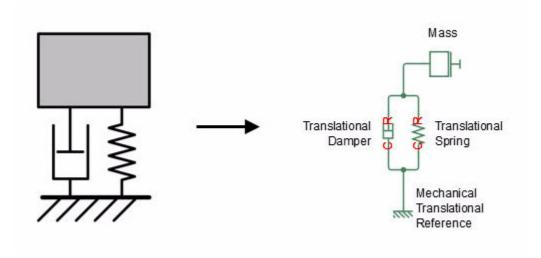
When constructing your network, it is important to include domain-specific reference blocks, such as Electrical Reference, Mechanical Translational Reference, and so on. Depending on domain, these blocks represent connection to ground, frame, or atmosphere. For more information, see "Grounding Rules".
